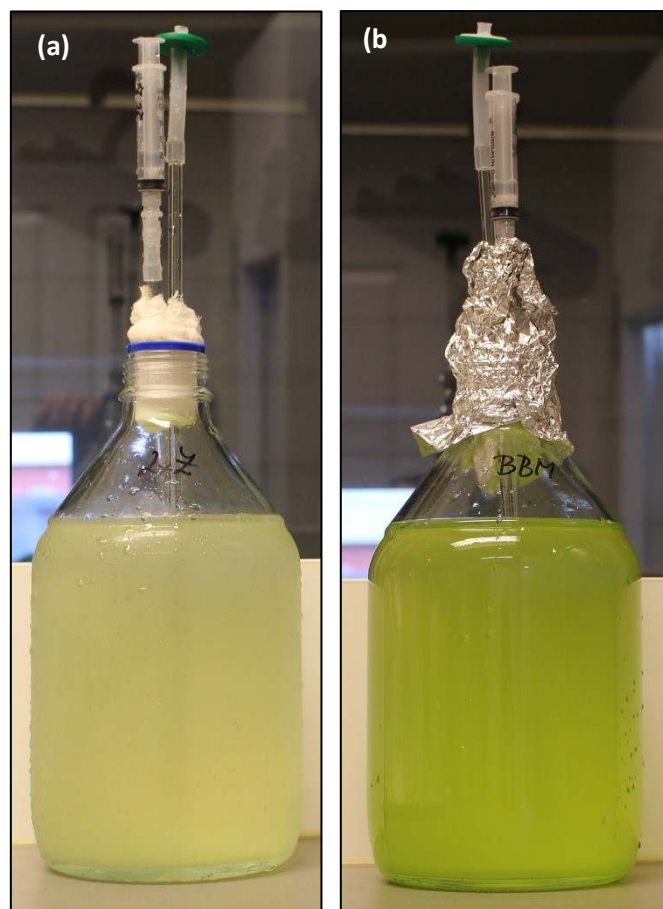
Fig. 3.2.7. The algal cultures in 2 l cultivation vessels before harvest grown in (a) 2xZ-medium 2 , (b) BBM medium 3 .
