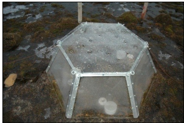
Fig. 3.4.11. The modified OTC - CTC in wet meadow, Petuniabukta, Svalbard.
