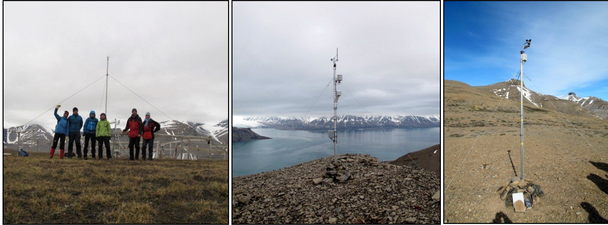
Fig. 3.2.2. Automatic weather stations in the vicinity of Petuniabukta (AWS1 – marine terrace, AWS4 – mountain ridge of the Mumien Peak, AWS8 – near the Fortet Peak).
